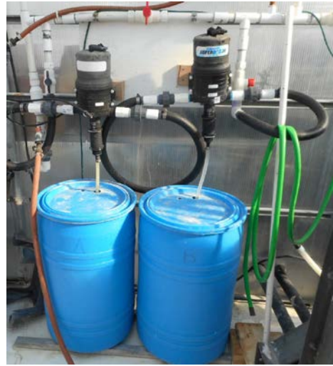
Two fertilizer stock tanks each with their own fertilizer injector are used because some fertilizer are incompatible with each other in concentrated amounts.
