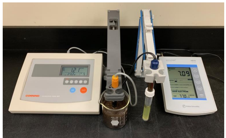
Figure 3. Examples of benchtop meters. In this scenario, separate electronic consoles are needed for pH and for EC, although many benchtop meters have the ability to measure both.
